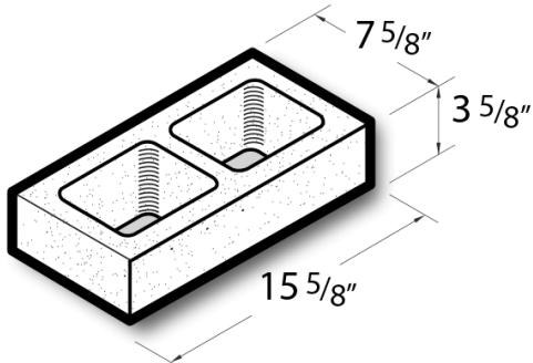
8x4x16 Best Brik™ CMU is a half high concrete masonry unit that offers the aesthetics of brick, while retaining the strength, durability, fire resistance, sound-proofing, energy efficiency, and affordability benefits of CMU. Ideal for partially or fully grouted single wythe walls or veneers. [Contact](#) your Best Block representative for special requests and additional options.
