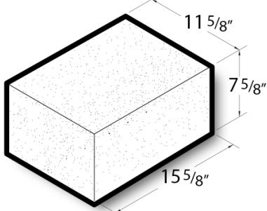
12x8x16 Solid Block is a standard concrete masonry unit (CMU) that exceeds ASTM C90 standard specifications in all weight classifications. [Contact](#) your Best Block representative for special requests and additional options.
