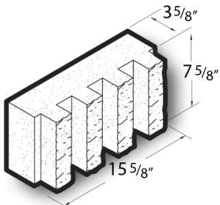
4x8x16 4 Rib Split or Ribbed block includes vertical scores and come in a wide variety of styles and sizes that exceed ASTM C90 standard specifications in all weight classifications. [Contact](#) your Best Block representative for special requests and additional options.
