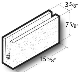
4x8x16 Bond Beam Block is a standard concrete masonry unit (CMU) that exceeds ASTM C90 standard specifications in all weight classifications. [Contact](#) your Best Block representative for special requests and additional options.
