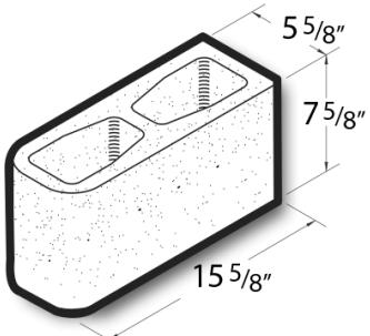
6x8x16 Double Bullnose Block is a standard concrete masonry unit (CMU) that exceeds ASTM C90 standard specifications in all weight classifications. [Contact](#) your Best Block representative for special requests and additional options.
