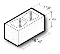
8x8x16 Double Jamb Pilaster Block is a standard concrete masonry unit (CMU) that exceeds ASTM C90 standard specifications in all weight classifications. Contact your Best Block representative for special requests and additional options.
