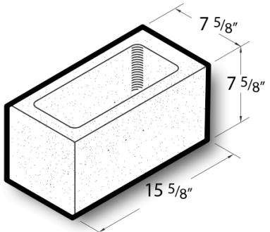
8x8x16 Single Core Pilaster Block is a standard concrete masonry unit (CMU) that exceeds ASTM C90 standard specifications in all weight classifications. [Contact](#) your Best Block representative for special requests and additional options.
