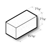
8x8x16 Solid Block is a standard concrete masonry unit (CMU) that exceeds ASTM C90 standard specifications in all weight classifications. Contact your Best Block representative for special requests and additional options.
